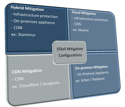
**Hybrid:** A hybrid solution is a combination of on premise mitigation box and remote cloud defenses. An on premise appliance provides defense against smaller volumetric attacks and application layer attacks. In volumetric attack situations, the cloud solution is able to divert the traffic into a scrubbing center before rerouting back to the customer network. True joint solutions have not been common. Cloud providers have been somewhat reluctant to move into the business of selling hardware.
